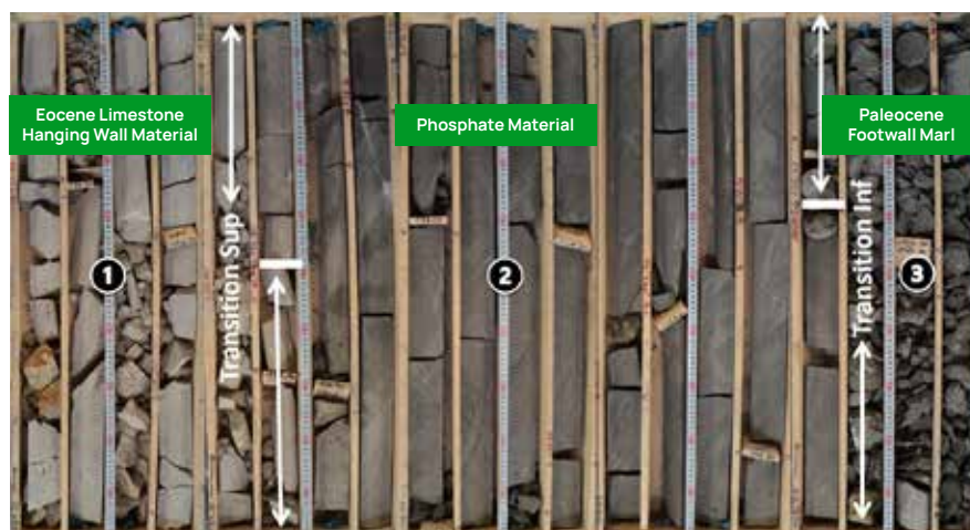
Figure 2.1 Typical Drill Core Lithological Section Chaketma Stratigraphy
